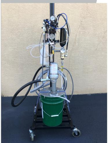
Systems are Built to Last Feature Stainless Steel Fluid Pumps System can be configured as External or Internal Mix Pump Output and Ratio: 1.5 GPM, 15:1
